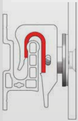
Hook system « free point » with anti-noise solution to avoid any noise pollution.
