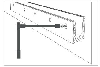
3 - Adjust and fix the rail with the appropriate wrench to the fixing pins.
