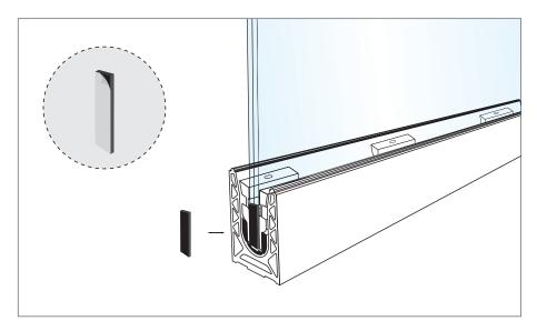
1 - Remove the protection from the adhesive. Stick the SADEV spacer on the edge of the glass, on the bottom right-hand corner flush with the glass.
