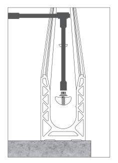
4 - Adjust and fix the rail with the appropriate wrench to the fixing pins.
