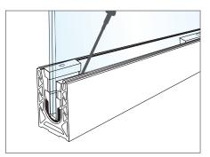
4 - Using a screwdriver, pry between the intermediate and upper wedge to remove the high wedge.
