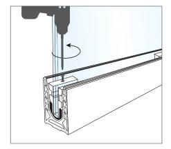
1 - After removing the cladding and gasket, unscrew the screws 1 cm high.
