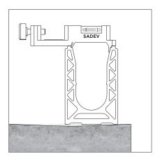
2 - Clip the specific levels on the profile, at a useful distance to put your level (see top view).
