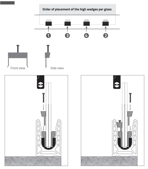
Insert the high wedge while maintaining the level of the glass
