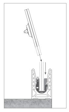
1 - Lift the glass inside the wedges.
