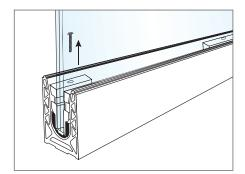
3 - Finish unscrewing the screw and remove it
