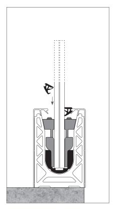
1 - Add the press-in gasket between the cladding and the glass.
