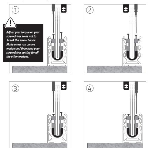
1 - Screw on each side of the glass as long as you do not change the level of the glass.
