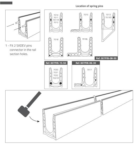
2 - Connect the rails together by using a mallet.
