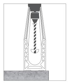
1 - Drill the support with a tool adapted to it.
