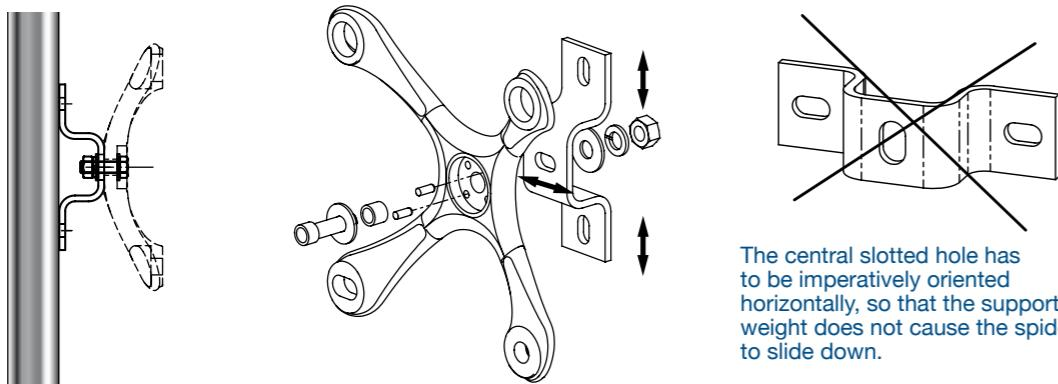
In order to obtain a correct adjustment of the spider, it is recommended to use an intermediary part, the "Omega". This part allows a bi-directional adjustment.
