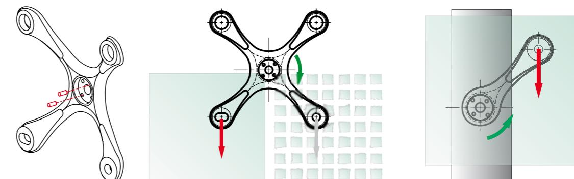
1 - In case of glass breakage, the spider is dragged in rotation by the remaining glass panel. It's from this point that the pins maintain the spider in position.
